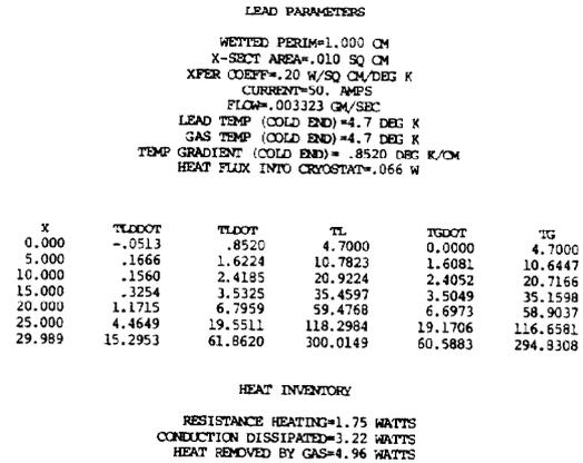
Fig. 3 Computed lead characteristics
