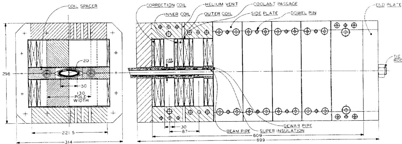
Figure 1. Cross section and elevation of the wiggler
