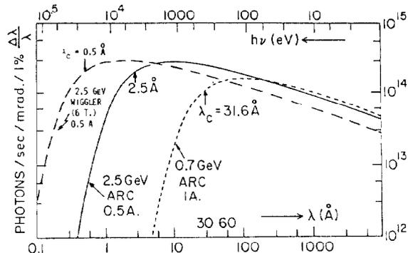
Figure 3. Spectrum of the synchrotron radiation emitted by the NSLS VUV and X-ray rings, and by the wiggler inserted in the X-ray ring.
