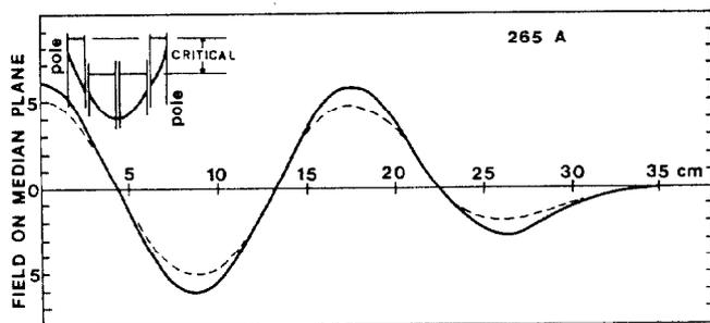
Figure 2. Calculated wiggler field on the median plane for 265 A. The field in the coils is also shown, together with the limiting field in the superconductor.
