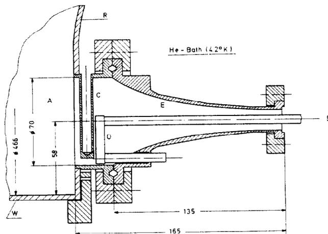
Fig. 3: Higher mode coupler. A: Cavity interior, B: Coaxial line, C: Field transformer, D: Coupling loop, E: Exponential line, R: Cavity endplate, W: Cavity cylinder wall
