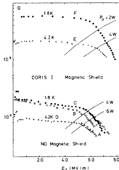
Fig. 1: Q<sub>0</sub> versus E<sub>p</sub> for runs A-F; cavity always kept under vacuum. Beside the improvement due to the magnetic shield all changes, especially the Q-jump in run B, are due to RF-processing
