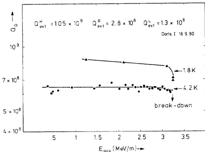
Fig. 2:  $Q_0$  versus  $E_{acc}$  measured in DORIS I after mechanical changes and with higher mode couplers
