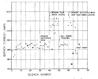
Fig. 2. Quench current versus quench number for the "D" bend dipole magnet.
