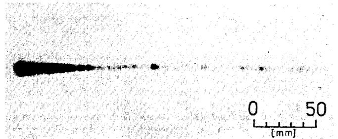
Fig. 7 Radiograph (Kodirex) taken from a septum electrode. This septum (49 molybdenum strips, 7 mm wide, 0.1 mm thick, spaced 1 mm apart) was used to split in half a 590 MeV, 12  $\mu\text{A}$  proton beam for a total of 20  $\mu\text{Ah}$ . The radiograph was taken 2 days after the septum was removed from the beam line. Dose rate at the entrance of the septum was 3R/hr. Time of exposure was 5 sec. Shown are the first 32 strips.
