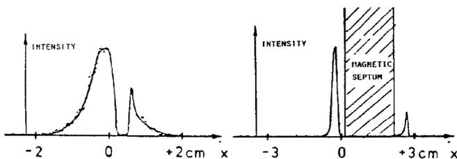
Fig. 6 Profiles of the splitted beam measured 0.5 m (left) and 5 m (right) after the splitter. The shaded area indicates the 20 mm thick septum coil of the bending magnet which separates completely the beam for the biomedical irradiation facility (small profile) from the main beam. At this point the beams are brought to two separate foci. The horizontal emittance of the unsplit 590 MeV beam is  $\pi \cdot 2.4$  mm mrad for 87% of the beam.
