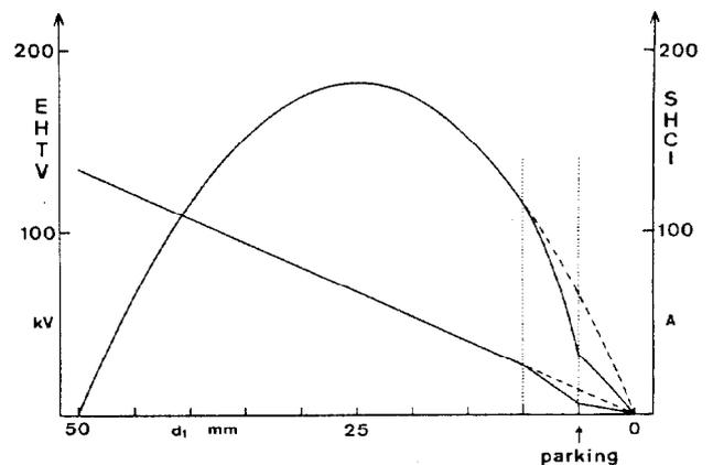
Fig. 5 Graphical representation of the parabolic relation between  $d_1$  and EHTV (common high voltage on the cathodes) and the linear relation between  $d_1$  and SHCI (current through the steering magnet SHC).
