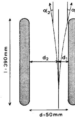
Fig. 4 Geometric parameters of the beam splitter. The distance between the two cathodes (dotted area) is constant. The sum of the two deflection angles  $\alpha_1$  and  $\alpha_2$  is constant and must not depend on the septum position.
