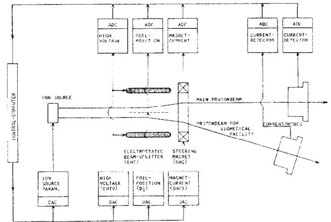
Fig. 3 Control diagram of the electrostatic splitter. Shown are the interconnections between the Control Computer and the parameters for setting (four) and checking (five) the splitter.
