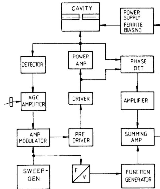
Fig.3 Block diagram of the amplitude and phase control
