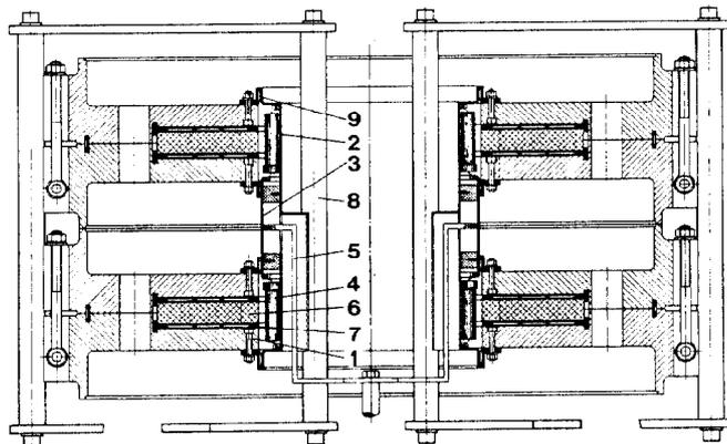
Fig.1: Cross section of the ferrite test-cavity
