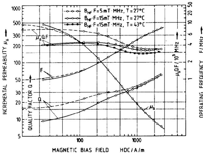
Fig.2: Data measured on FXC 8C12 rings (No.10/12)
