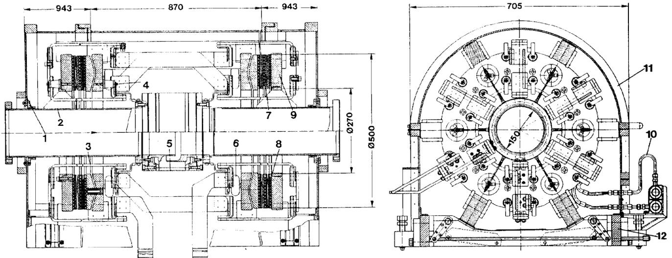
Fig.4: Cross-section of the prototype accelerating cavity built at GSI
