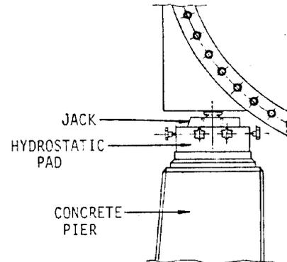
Fig. 9. Jack and pads on the support piers.
