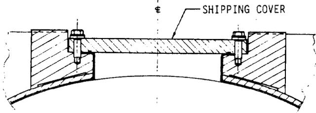
Fig. 3. Girder - drift-tube port.
