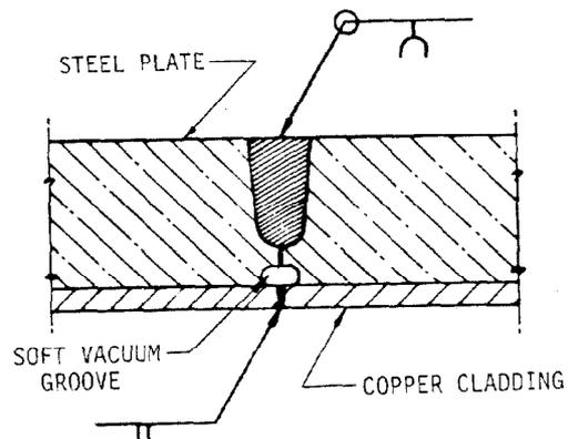
Fig. 2. Tank circumference weld seam.
