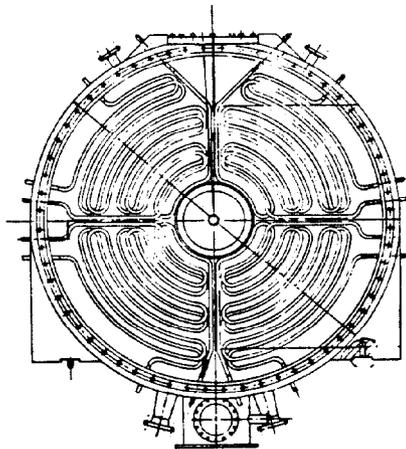
Fig. 7. Tank end-wall cooling.
