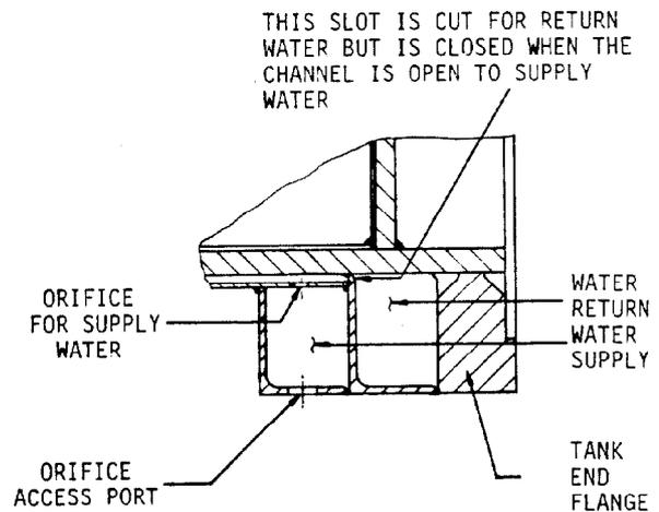
Fig. 6. Tank shell water system.
