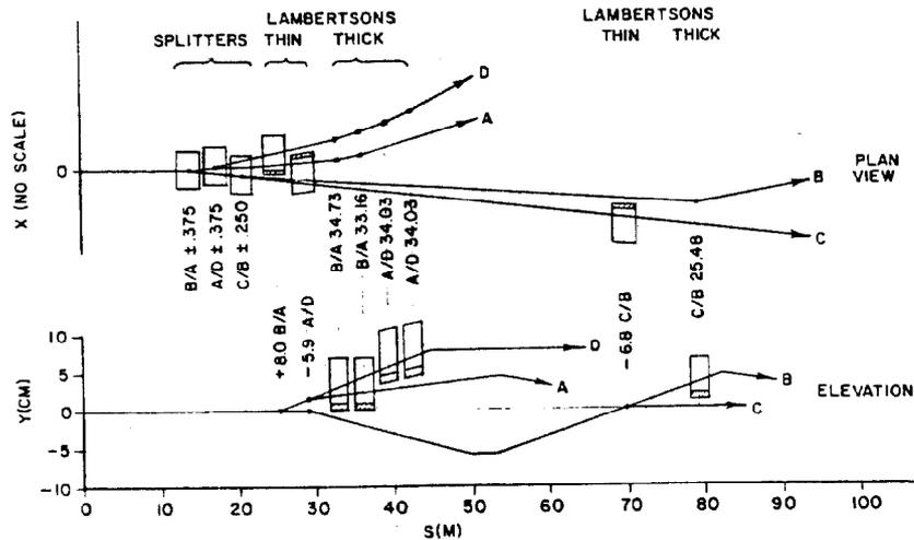
Fig. 4. Schematic Beam Splitting Layout. The Lambertson magnets are outlined to show their septum placements; they deflect in the opposite plane. Deflection angles are shown in milliradians.
