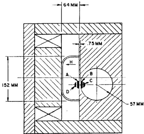
Fig. 2. Thin Lambertson Septum Magnet Cross-Section. This septum lies in the shadow of the splitter of Fig. 1. The D,A beams are deflected up.
