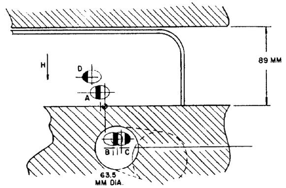
Fig. 3. Thick Lambertson Septum Magnet Cross-Section. This septum lies between the beam segments separated by the magnet of Fig. 2. The D,A beams are deflected to the left.
