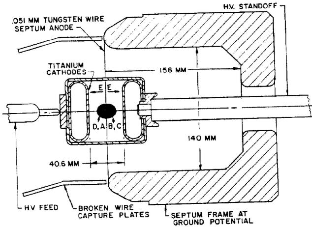
Fig. 1. Electrostatic Splitter Cross-Section. Typical placement for the D,A/B,C split. The D/A and B/C splits are made in succeeding splitters.
