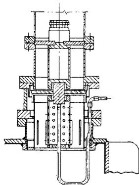
Figure 3. Coupling Loop and Vacuum Window.
