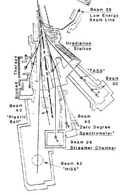
Figure 2 - Bevatron/Bevalac Experimental Area. Same - pulse beam sharing is possible between one beam line to the left of, and one to the right of the (imaginary) sharing axis.
