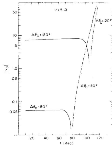
Fig. 2. Voltage at the end of the rf cycle on the capacitor versus  $T_1$ . Interval  $T_3$  is the parameter. The solid lines indicates positive voltage, the dashed lines indicates negative voltages.
