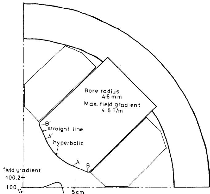
Fig. 4 Pole shape and calculated field gradient of quadrupole magnet.
