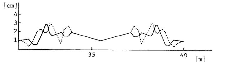
Fig. 3 Beam envelopes along LEPBT.
