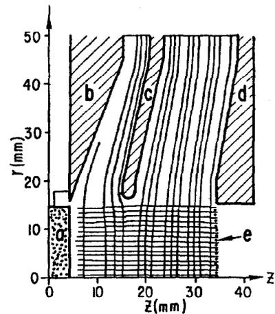
Fig. 4. Electrode Structure for the Cs<sup>+</sup> Gun: (a) Cs<sup>+</sup> Ion Emitter; (b) Beam Forming Electrode; (c) Intermediate Electrode; (d) Final or Ground Electrode; (e) Grid.
