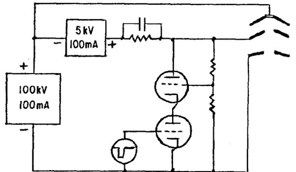
Fig. 5. Schematic of the Cs<sup>+</sup> Gun Power Supply
