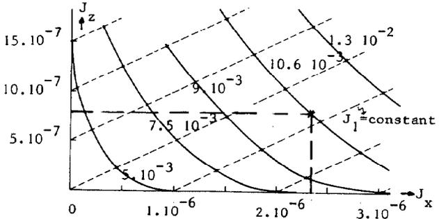
Figure 3.  $\delta Q/|F|$  curves in the  $J_x, J_z$  diagram for the resonance  $2Q_x + Q_z = p_r N$
