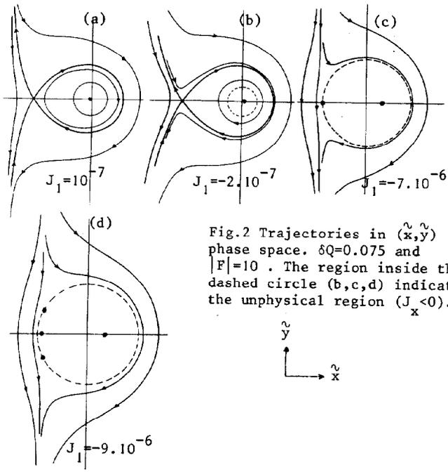
Fig.2 Trajectories in  $(\tilde{x}, \tilde{y})$  phase space.  $\delta Q = 0.075$  and  $|F| = 10$ . The region inside the dashed circle (b,c,d) indicate the unphysical region ( $J_x < 0$ ).
