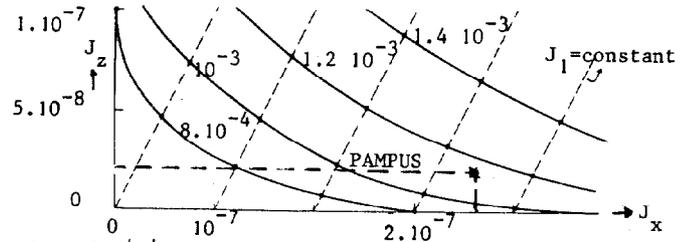
Fig.5  $\delta Q/|F|$  curves as function of  $J_x, J_z$ ;  $\delta Q = \frac{1}{2}(Q_x + 2Q_z - p_r N)$
