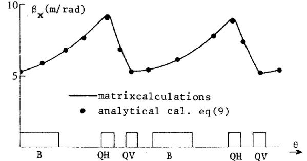
Figure 1. Behaviour of radial betatronfunction for PAMPUS with  $Q=2.10$
