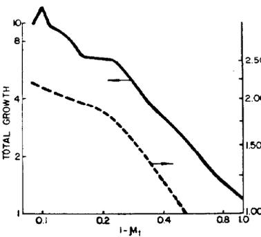
Fig. 2. Emittance growth in 72-cell, constant  $\sigma_0 = 50^\circ$ , constant  $E_0$  drift-tube linac;  $(\epsilon_t/\epsilon_\ell)_{\text{initial}} = 5.65$ .
