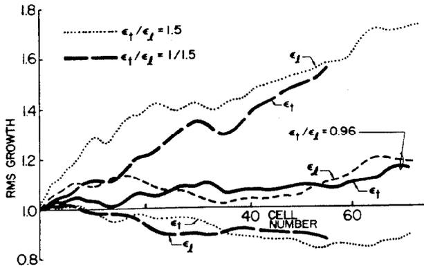
Fig. 4. Rms emittance growth in 72-cell, constant  $\mu^t = 0.9$ , constant  $E_0$  linac. Initial  $\mu^2 \sim 0.8$ .
