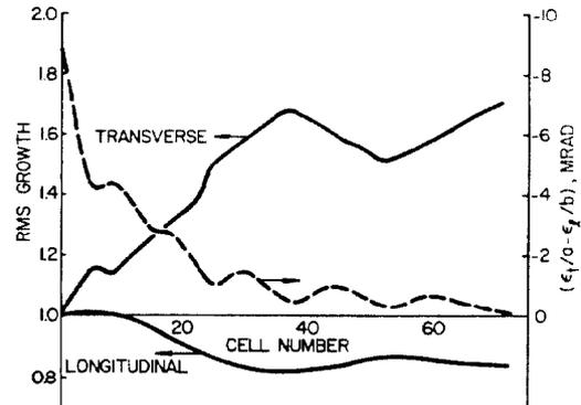
Fig. 3. Rms emittance growth and  $(\epsilon_t/a - \epsilon_l/b)$  in constant  $E_0$  linac. Initial  $\mu^t \sim 0.75$ ,  $\mu^l \sim 0.55$ ,  $\epsilon_l/\epsilon_t = 5.65$ .
