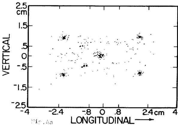
Fig. 4 a. scatter plot of 512 UV initiated events. b. histograms of data in a.
