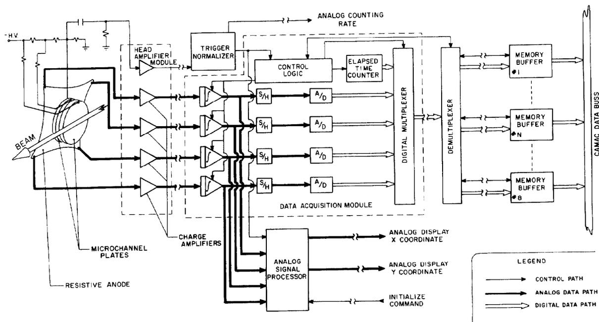
Fig. 5 PROFILE MONITOR SIGNAL PROCESSING DIAGRAM
