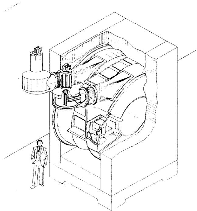
Fig. 4. The superconducting coils are in separate cryostats which occupy the same space used by the present aluminum coils.
