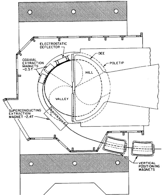
Fig. 7. The beam extraction system for the conversion. The two vertical positioning magnets are to be provided with coils to compensate the effect of the stray field on the iron yokes.
