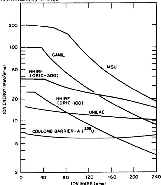
Fig. 1. Energy vs. mass characteristics for the ORIC in present coupled operation with the 25 MV tandem (ORIC-100), and for the conversion (ORIC-300), for beam intensities of  $10^{11}$  particles/sec. Energy characteristics of other large facilities are shown.
