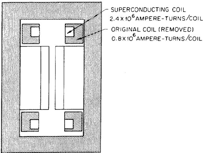
Fig. 2. The superconducting coils will have a smaller cross-section than the present coils and are effectively nearer the median plane and of larger radius.
