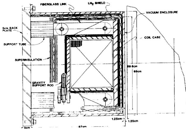
Fig. 5. Cross-section of the cryostat/coil assembly.
