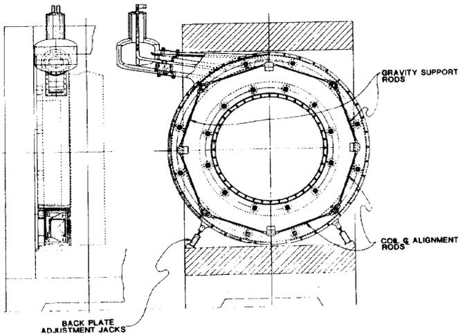
Fig. 6. Side-view of the cryostat/coil assembly showing the coil centering supports, alignment system, and coil leads.
