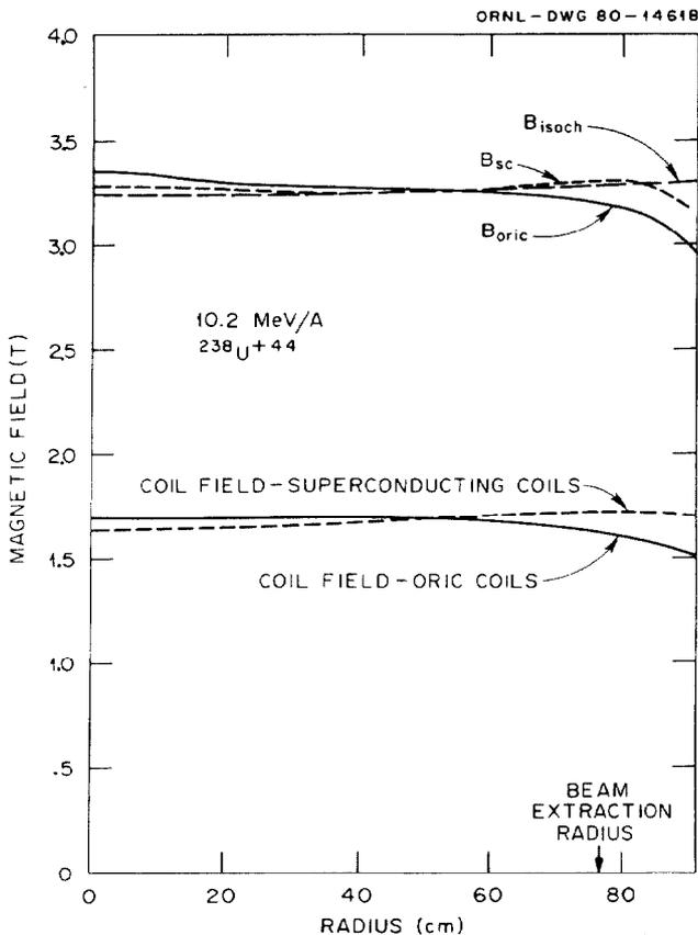
Fig. 3. Radial profile of average magnetic field for the conversion showing the improvement in shape obtained with optimized coil geometry.
