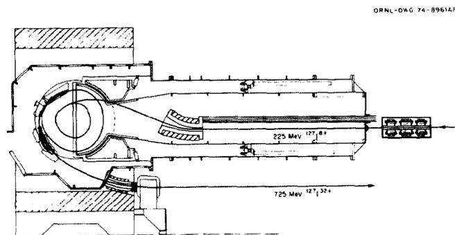
Fig. 1. Beam enters the cyclotron through the rf resonator, is directed by the inflection magnet to the stripping foil which is placed on an orbit suitable for acceleration. The incoming beam must have a sufficiently large rigidity ( $B\rho$ ) to cross the field to the foil. The inflection magnet is movable radially and has an angular range of 17 to 37 deg to accommodate beams of different rigidity requiring different deflection angles.
