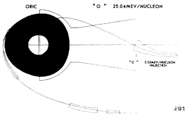
Fig. 5. Calculated injection, acceleration, and extraction trajectories for the 400 MeV  $^{16}\text{O}^{8+}$  beam. The program finds the optimum positions for the foil and the inflection magnet. The operator iteratively adjusts the positions and strengths of the five extraction elements to achieve the desired calculated result, in a manner similar to actual operation.
