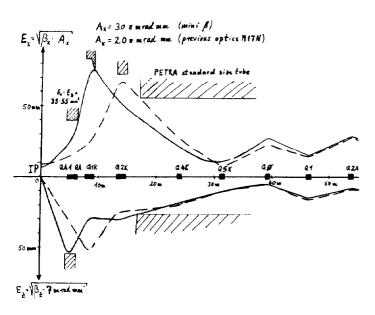
Fig. 3: Horizontal and vertical envelopes near the interaction point
