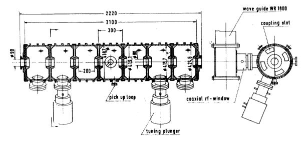
Fig. 1: PETRA new type 7-cell acceleration cavity (500 MHz)
