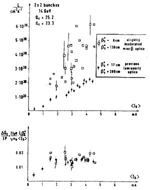
Fig. 4: Comparison of measured luminosity and vertical linear tune shift at 14 GeV with 2x2 bunches as a function of bunch current  ${\rm I}_{\rm h}$
