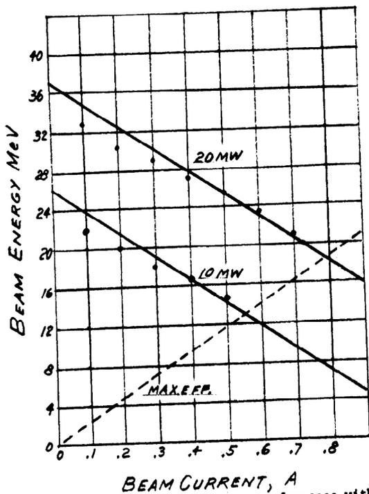
Fig. (2) Theoretical Steady-State performance with experimental data indicated.
