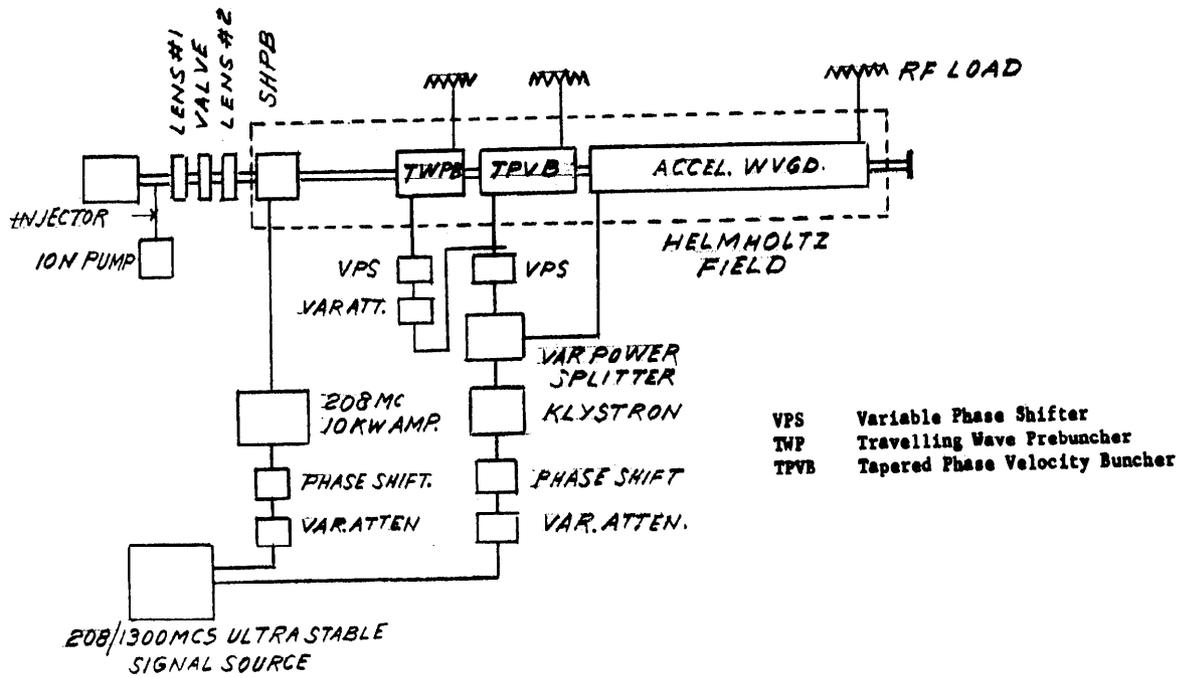
Fig.(1) Diagram of Major Components of ISIR Linac
