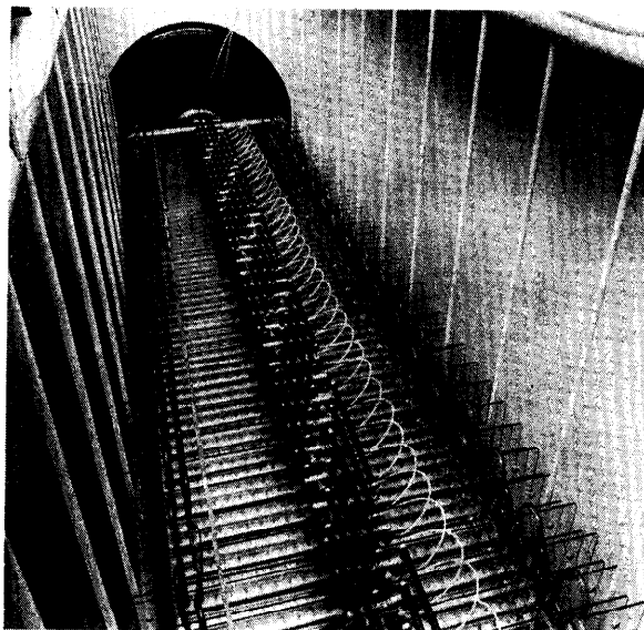
Figure 3 Modular Marx generator suspended in tank with compact stages connected by charging and triggering resistors.
