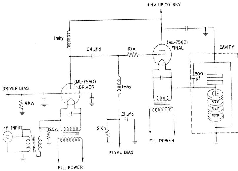
FIG. 1 SCHEMATIC DIAGRAM DEMONSTRATION AMPLIFIER
