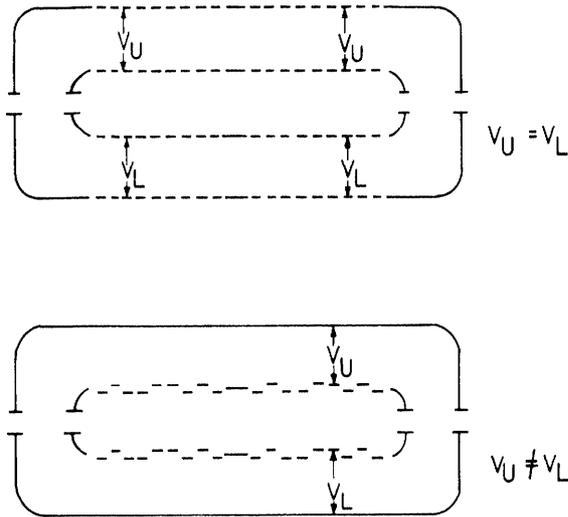
Fig. 5. Outline view of a dee as seen from the accelerating gap. (a) Resonators ideally aligned, (b) resonators realistically aligned.
