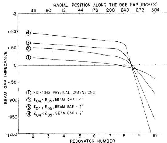
Fig. 3. RF impedance of the beam gap along the dees.
