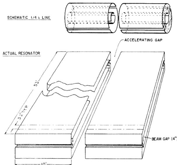
Fig. 4. The TRIUMF resonator derived from a simple quarter-wave stub.
