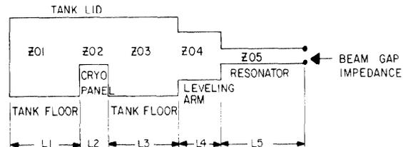
Fig. 2. Schematic cross-section of upper and lower structures.
