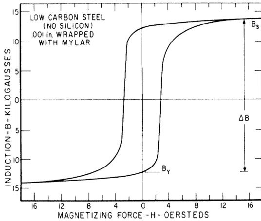
Fig. 4. Typical hysteresis curve for magnetic tape wound induction accelerator cores. During pulsing the total available change in magnetic induction  $B$  is from  $B_r$  to  $B_s$ . Between pulses the core must be reset to  $B_r$ .
