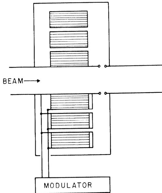
Fig. 8. Illustration of radical stacking of induction accelerator cores driven by a single modulator.
