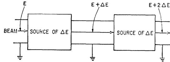
Fig. 2. Illustration of modular nature of induction linear accelerators, allowing repeated increments of energy gain while maintaining the space between modules at ground potential.
