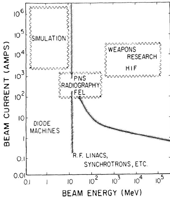
Fig. 1. Schematic illustration of the limitations of conventional accelerator technologies and the parameter needs of some accelerator applications. Diode machines operate to the left of the dashed line at about 15 MeV. RF linacs, synchrotrons, etc. operate below the dashed line of a few amperes or less. PNS indicates pulsed neutron source, FEL--Free electron laser, HIF--heavy ion fusion.
