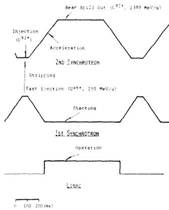
Fig.2 Operation Scheme of the Accelerator Complex
