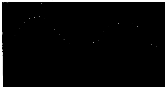
Fig. 6. Spatial profile monitor signal: horizontal profile is at left of photo and vertical profile is at right.
