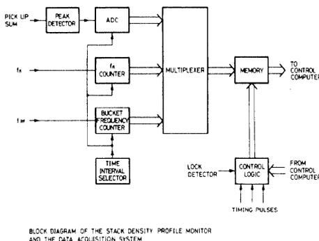
Fig. 3 The local data acquisition system and the density profile monitor
