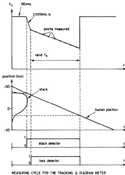
Fig. 2 A typical measuring cycle
