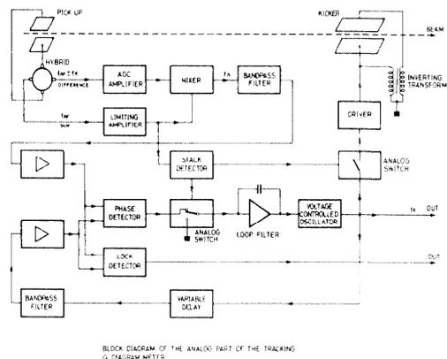
Fig. 1 Block diagram of the analogue part
