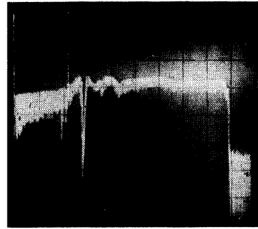
Photo 2 Excitation during whole accelerator cycle. Amplitude tracking of excitation loop at 18.5 \pm 1.5 kHz Rms amplitude 10 dB/div versus time 500 ms/div Log ref: -10 dBm \approx 2 mm Trigger at first injection Note injection oscillations at t_1 = 0 , t_2 = 1.2 s. Oscillation disappears at transition t_3 = 1.4 s and above 380 GeV t_4 = 4.5 s.
