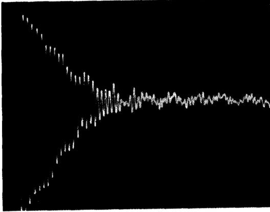
Fig.3b: Bunch oscillations with feedback. The time base is expanded by a factor 50 (0.2 ms/div)
