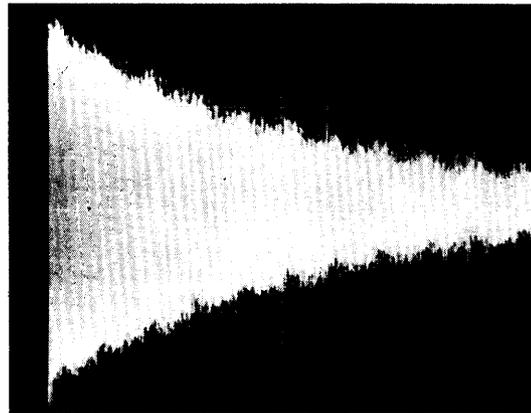
Fig. 3a: Coherent horizontal bunch oscillations without feedback (time base: 10 ms/div)
