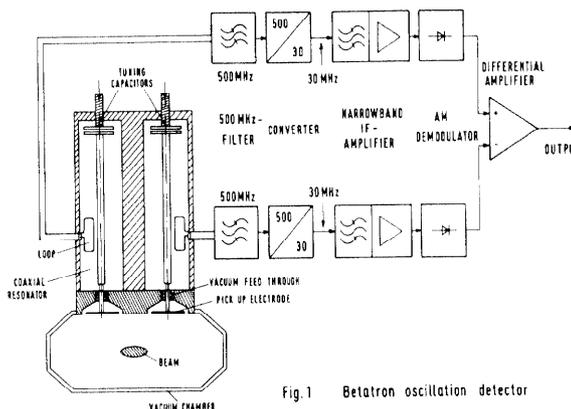
Fig.1 Betatron oscillation detector
