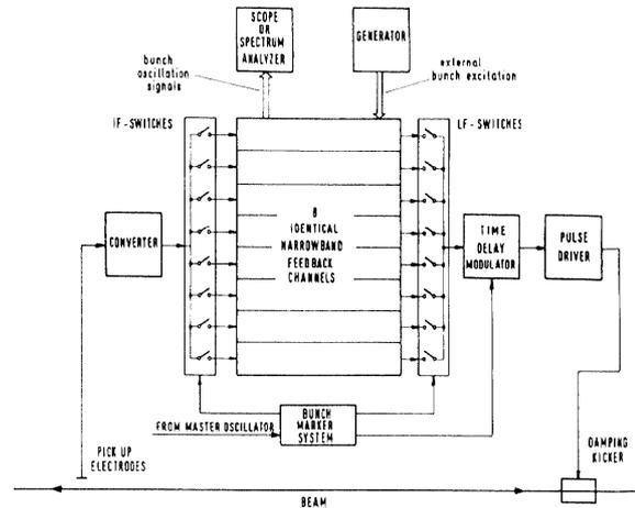
Fig.2 Arrangement of the 8channel feedback system
