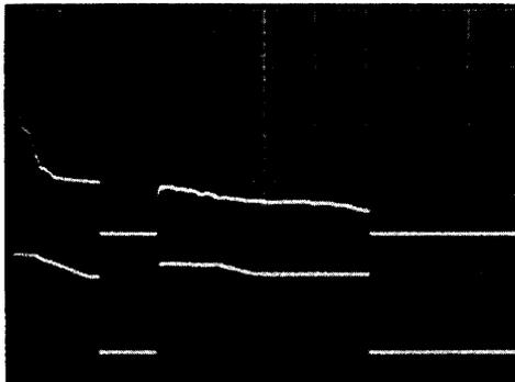
Fig. 2. Beam Intensity and RF Voltage Profile. The upper trace shows the beam intensity as measured by an ac detector during the acceleration cycle. The lower trace is the accelerating RF voltage during the acceleration cycle.
