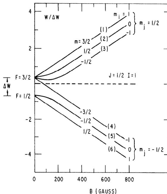
Fig. 1. Magnetic splitting of the hyperfine states of the deuterium atom  $\Delta W/h = 327.3843$  MHz.
