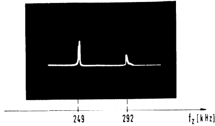
Fig. 5 Splitting of the vertical betatron frequency due to the beam-beam interaction (energy E = 4.6 GeV f_0 = 1041 kHz)
