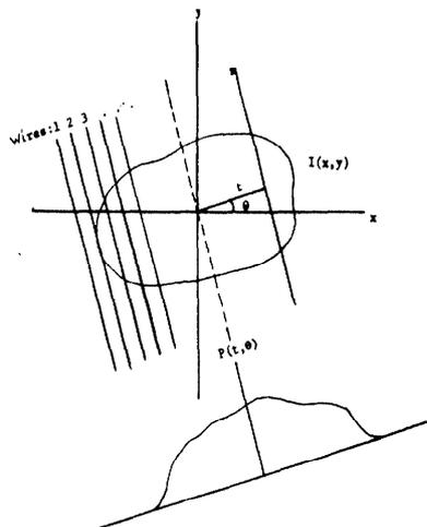
Fig. 1. Schematic diagram showing one of the sixteen signal wire planes and its projection of the actual beam profile, superimposed on the coordinate system used in reconstruction (see appendix). (XBL 793-8921)
