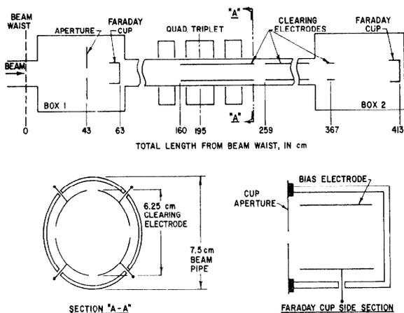
Fig. 1: Experimental setup, clearing electrode and cup details
