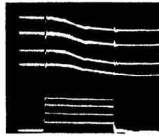
Fig. 6: Multiple exposure. Four beam traces for four clearing pulses of different amplitudes. Top beam trace (1 mA/div.) corresponds to top pulse trace (100 V/div.), etc. Current trace to trace for clarity. End of pulse indicated by Time base 2  $\mu$ s/div.
