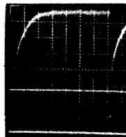
Fig. 8: Beam current  $\sim 1$  mA (0.2 mA/div.). Pulse width 6  $\mu$ s height 100 V. Higher vacuum.
