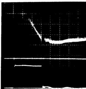
Fig. 5: Typical beam response to a +200 V, 6  $\mu$ s pulse. From top to bottom: 1st trace-beam current 0.2 mA/Div., 2nd trace-base line for the beam current, 3rd trace-clearing pulse 100 V/Div., 4th trace-base line for the clearing pulse.
