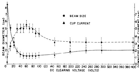
Fig. 4: Measured beam size and current for different values of clearing potential.
