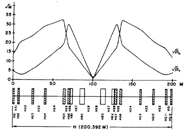
Fig. 6 High-luminosity insertion H.
