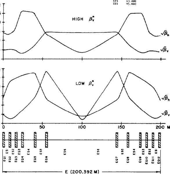
Fig. 5 General-purpose experimental straight-section insertion E.
