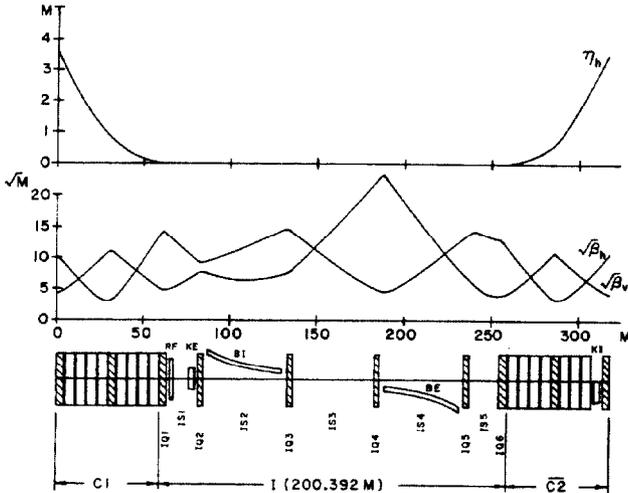
Fig. 3 Injection straight-section insertion I, together with cell C1 and C2, showing injection, stacking, and ejection elements.
