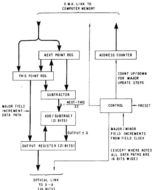
Fig. 2. Digital function generator interpolation logic
