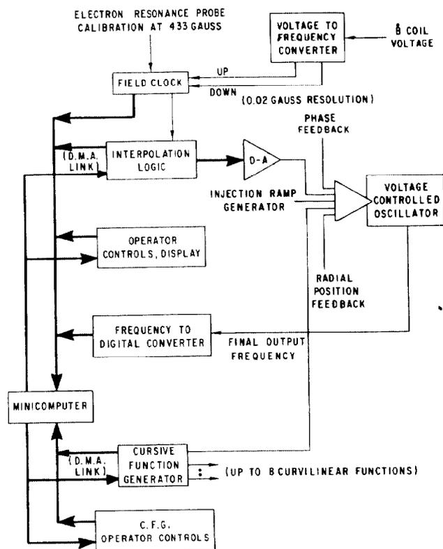
Fig. 1. Computer based RF control system block diagram
