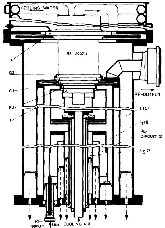
Fig. 6: mechanical design of the power stage
