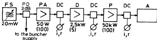
Fig. 1: block-diagram of the amplifier chain.
