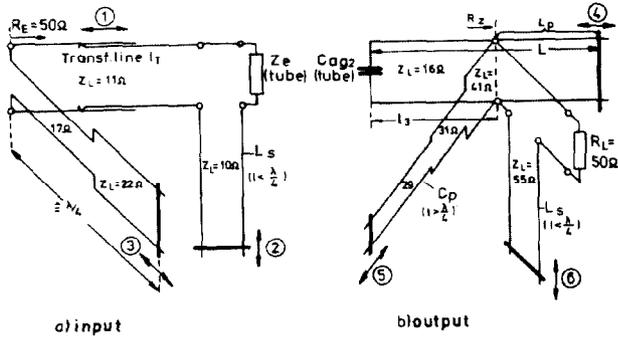
Fig. 3: equivalent diagram of the line circuitry.
