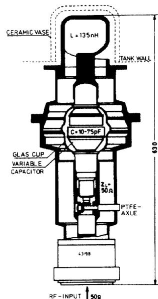
Fig. 8: capacitive compensated coupling loop.
