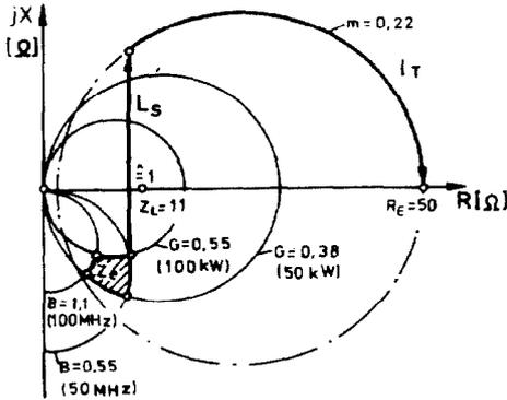
Fig. 4: input transformation in the impedance plane.
