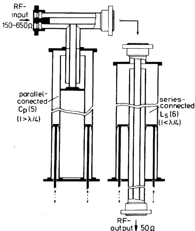
Fig. 7: mechanical design of the matching stubs.
