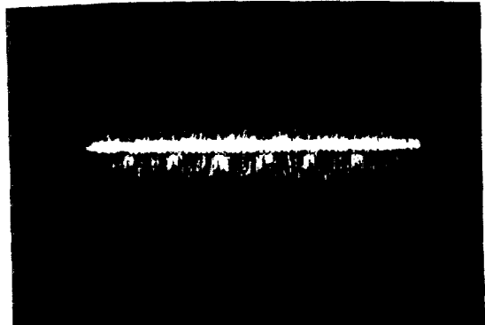
Fig. 4 The radial position signal shown here indicates bunch-by-bunch radial instabilities.
