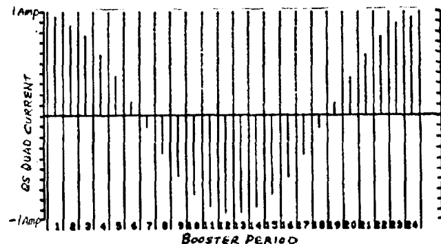
Fig.1 DC quad currents at period short straight sections for 1st harmonic correction with 0^\circ phase advance.
