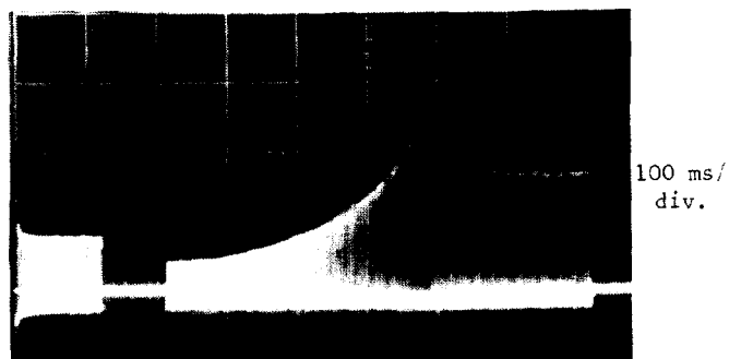
a) Wide-band pick-up station signal gap in signal waveform corresponds to coasting beam during harmonic number switching
