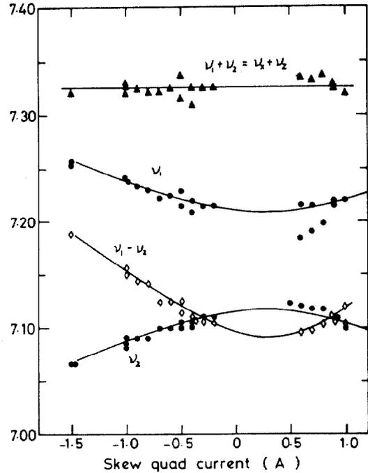
Fig.3 Two frequency components appearing in the vertical coherent oscillation signal when kicked horizontally.
