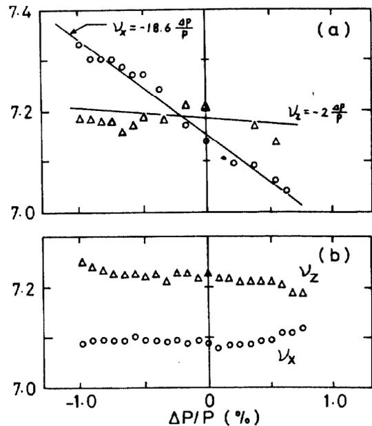
Fig.1 Chromaticity of the main ring. (a) uncorrected, and (b) corrected with F-sextupole of 2.0 A and D-sextupole of zero current.
