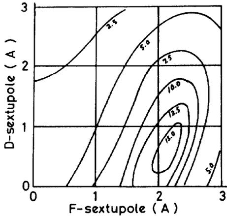
Fig.2 Intensity map in the diagram of F-sextupole and D-sextupole current.
