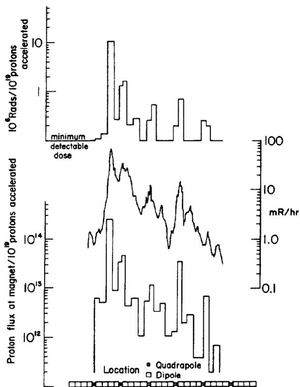
Fig. 3 Dose radiation survey and particle fluxes in A Sector for period of operation of Fig. 2.
