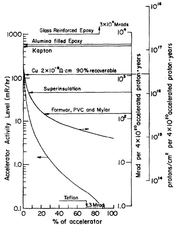
Fig. 4 Anticipated material property degradation for the Energy Doubler/Saver based on present accelerator operation.
