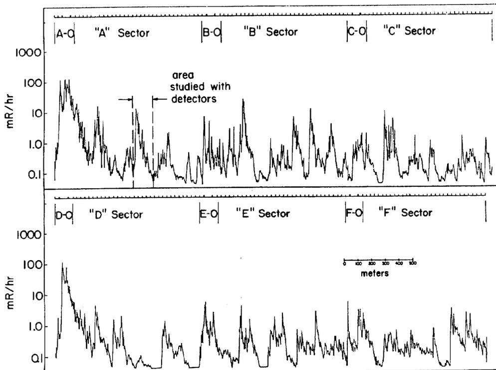
Fig. 1 Radiation survey of Main Ring one-half hour after beam turned off.
