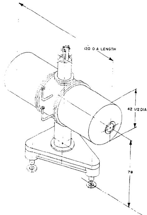
Fig. 1. Physical dimensions of the HEUB dipoles (in.).
