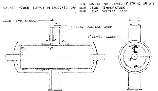
Fig. 5. The location of the instrumentation sensors on each magnet.
