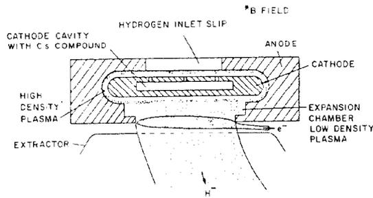
Fig. 6. Cross Section of the BNL  $H^-$  Magnetron Source. (Courtesy of Dr. Krsto Prelec - BNL)
