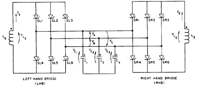
Fig. 7. Circuit Diagram for a Three-Phase Inductor-Converter Bridge.
