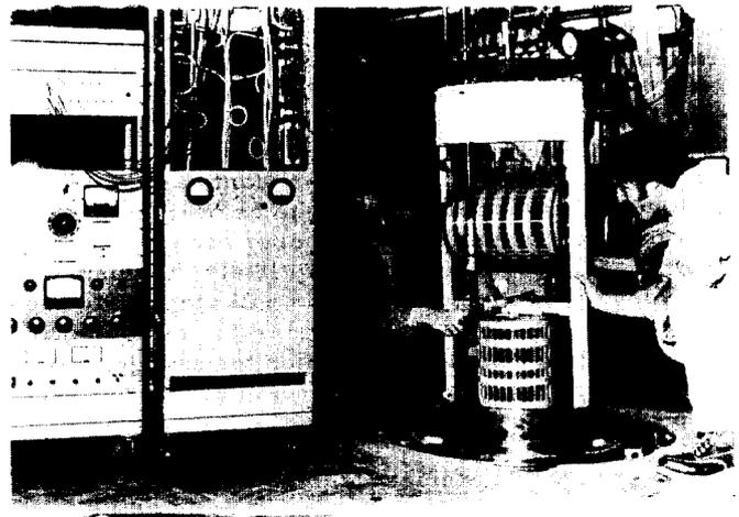
Fig. 8. Photograph of Test Model for Transferring Energy Between Two Superconducting Coils with Different SCR Bridge Circuits.
