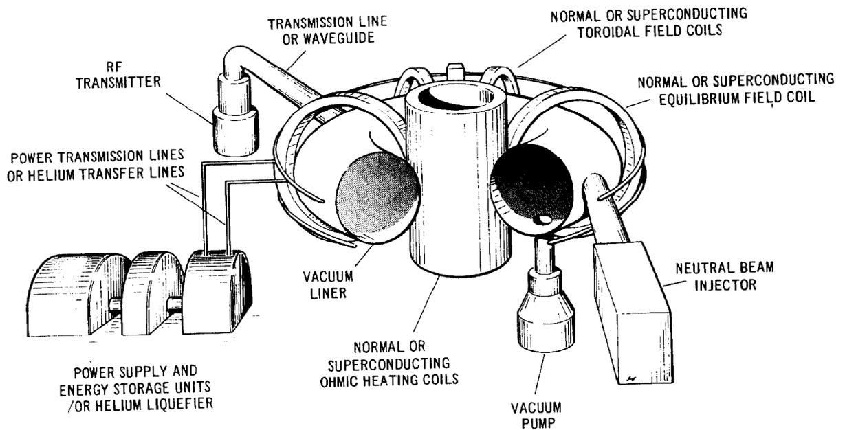
Fig. 2. Cartoon Version of a Tokamak Highlighting Major Subsystems
