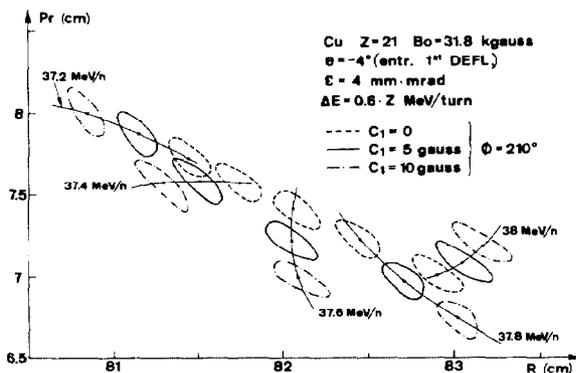
Fig. 3. Radial phase plots of an accelerated beam, without 1st harmonic, and with 5 and 10 Gauss 1st harmonic amplitude.
