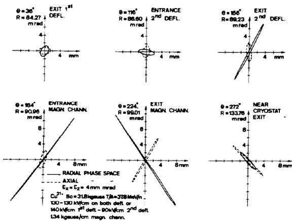
Fig. 5 . Radial (continuous line) and axial (dotted) phase space behaviour for a Cu 21+ beam of 37.8 MeV/nucl., at the various points indicated, along the trajectory of fig. 2.
