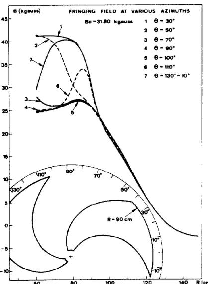
Fig. 1. Radial behaviour of the fringing field, at different azimuths, at a level of 31.8 Kgauss.
