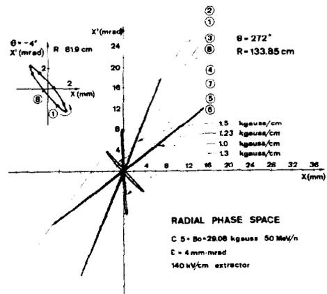
Fig. 4. Effect of different gradients of the magnetic channel on the radial phase space of the extracted beam as observed near the exit from the cryostat.
