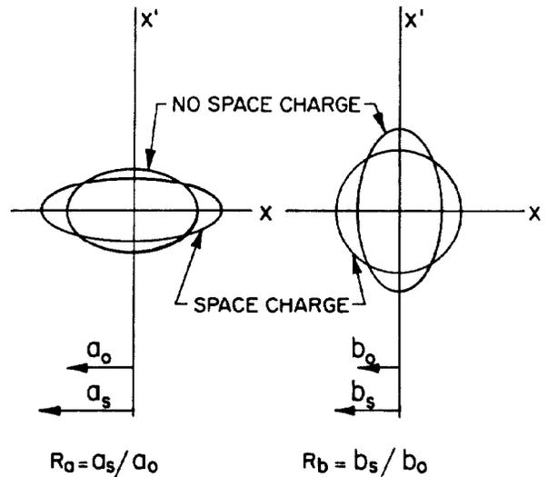
Fig. 1. Matched  $xx'$  phase space ellipses at the center of focusing and defocusing quadrupoles with and without space charge
