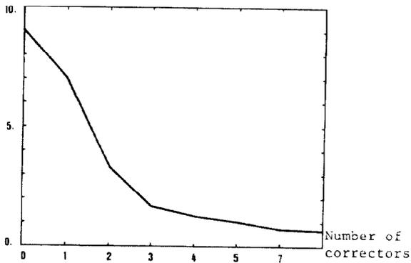
Fig. 1 : Maximum orbit deviations (mm)
