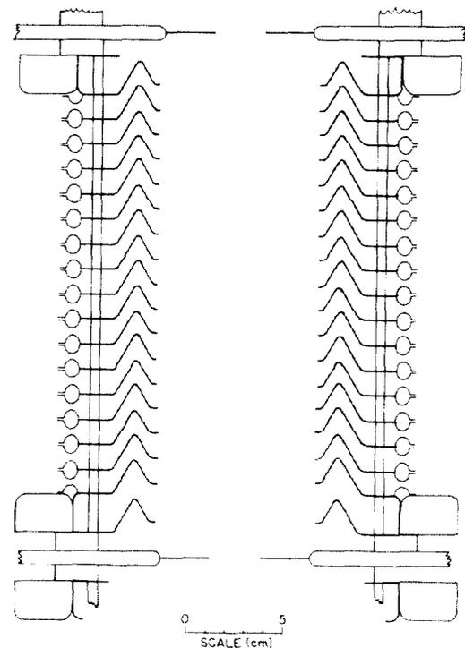
Fig. 1. A schematic cross section of a section of the accelerator tube and two decoupling sections.
