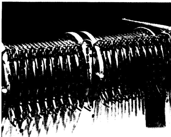
Fig. 3. A section of the voltage divider as it is attached to the accelerator tube.
