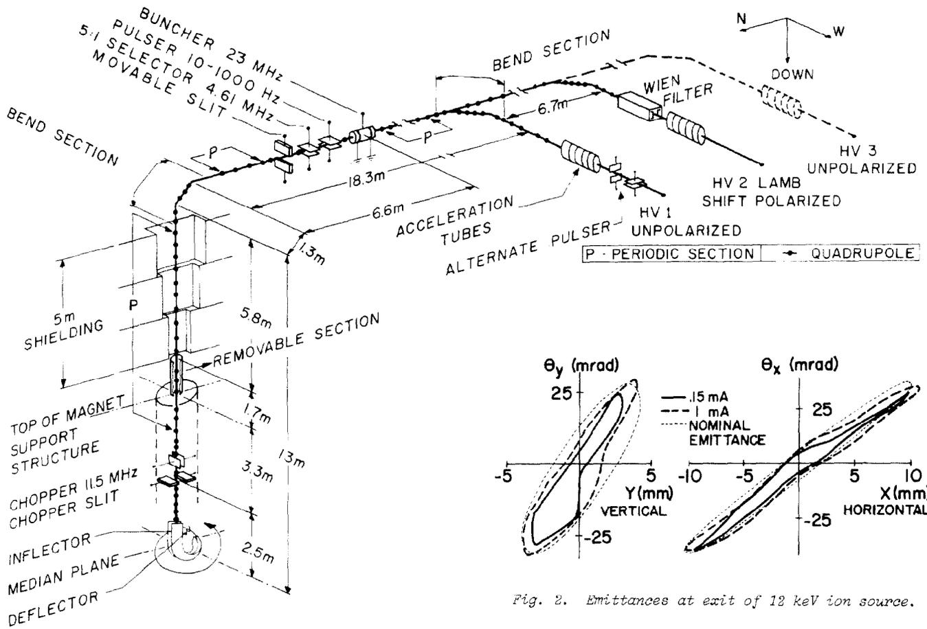
Fig. 1. Injection line layout.
