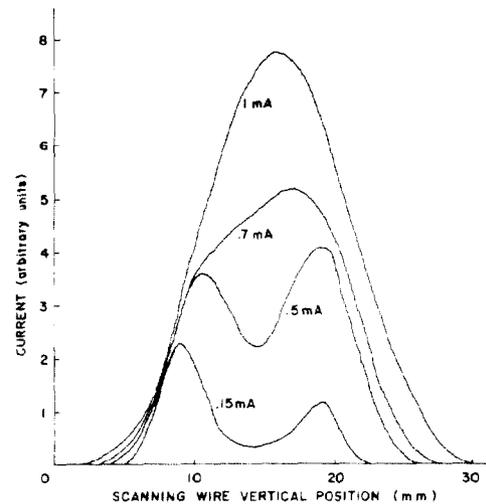
Fig. 3. Vertical beam profile at 12 keV ion source exit.
