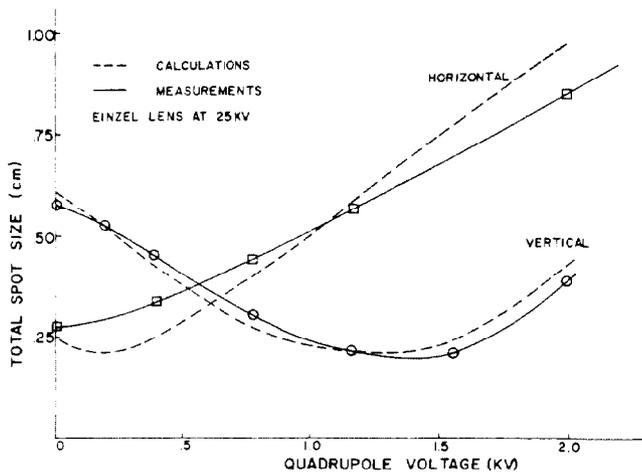
Fig. 4. Comparison of theoretical and measured 12 keV beam spot sizes.
