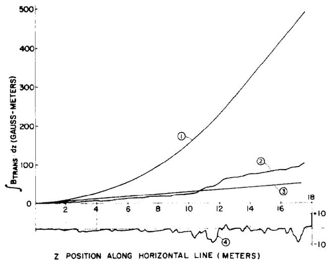
Fig. 5. Magnetic fringe field compensation. 1) Uncompensated field; 2) Field with mild steel shields; 3) Equivalent correcting power of electrostatic steering; 4) Field with mild steel shields plus optimized distribution of dipoles.
