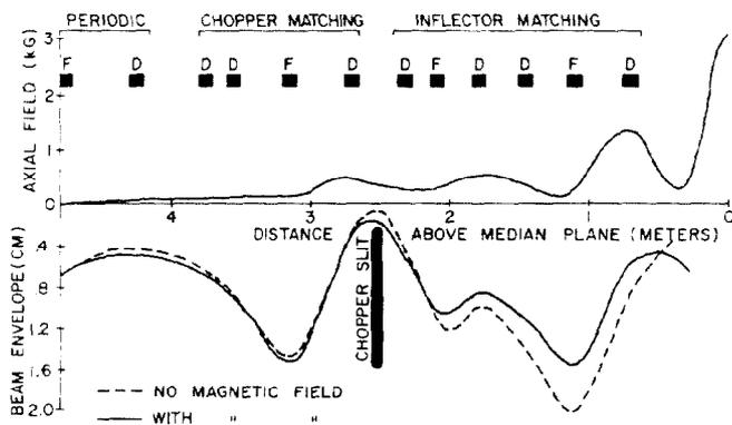
Fig. 6. Effect of cyclotron fringe field on beam envelope near chopper slit.
