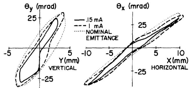
Fig. 2. Emittances at exit of 12 keV ion source.
