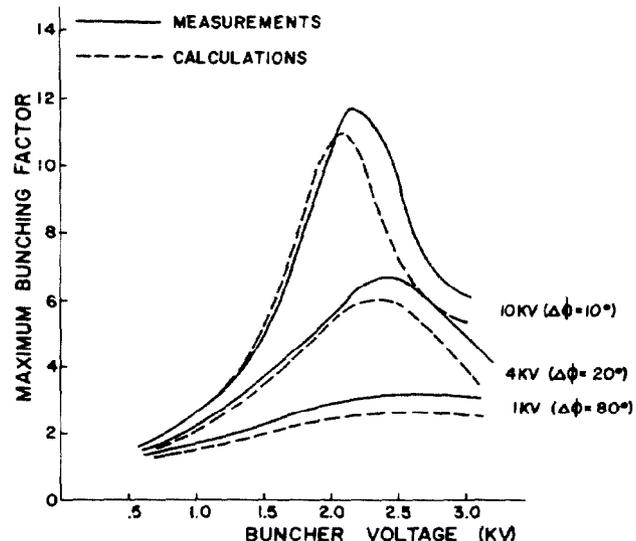
Fig. 7. Effects of bunching on beam transmitted through chopper slits, with phase acceptance and chopper peak voltage as parameter.
