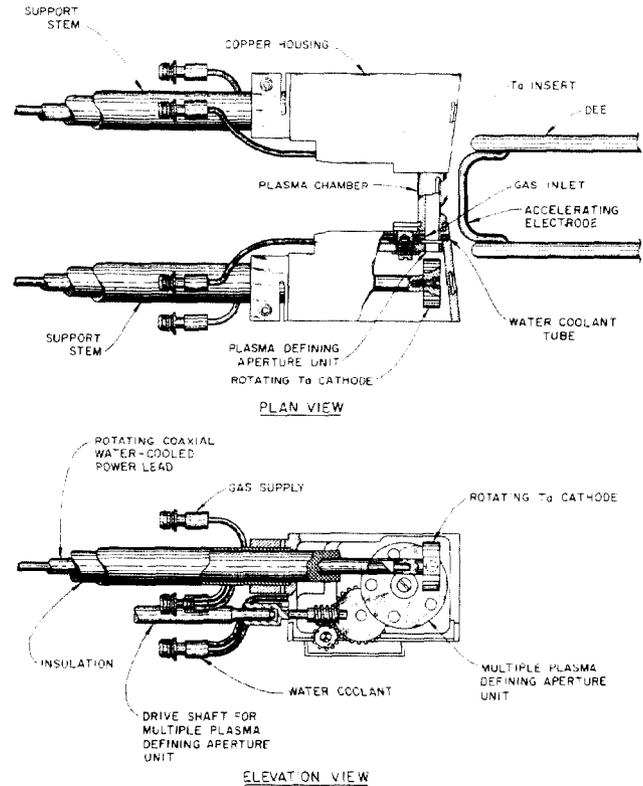
Fig. 1. A schematic drawing of the source head of the rotatable cathode ion source. The cathodes can be rotated and the plasma collimator has multiple apertures which can be changed remotely.
