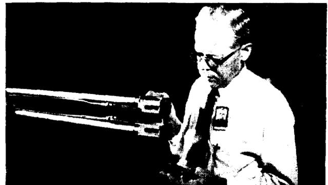
Fig. 2. The rotatable cathode ion source head. Normally located in the center of the cyclotron, the source head is mounted on a dual-stem structure that contains the drive shafts for the rotatable cathodes. The source head has many access ports with covers for quick maintenance.
