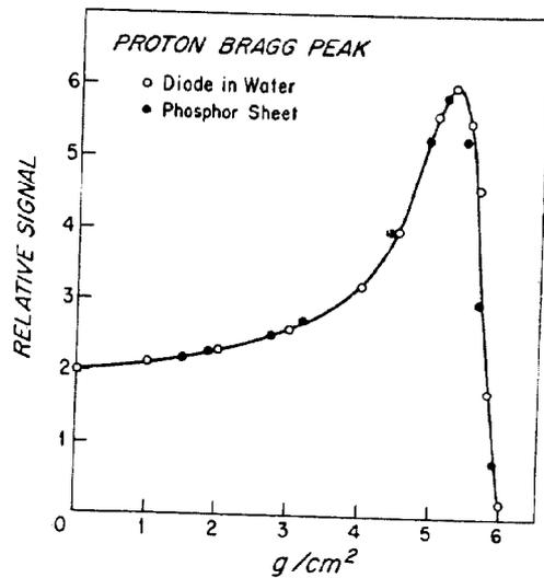
Fig. 5. Proton Bragg peak measured with a diode in water and with phosphorescence.
