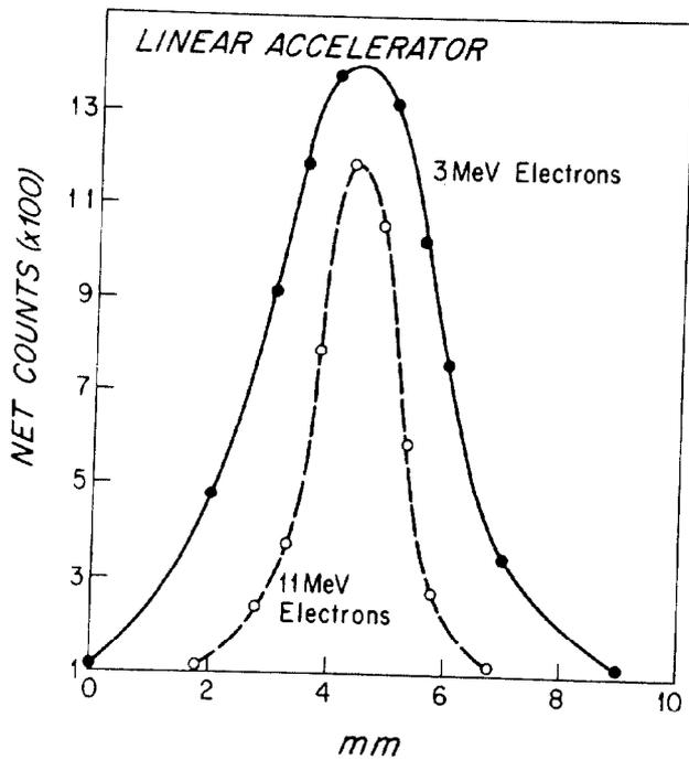
Fig. 2. Beam profile at the exit window of a linear accelerator.
