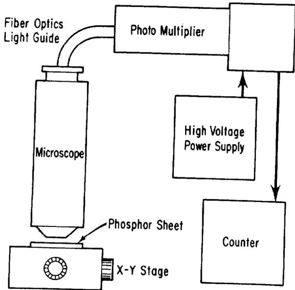
Fig. 1. Block Diagram of the phosphorescence scanning apparatus.
