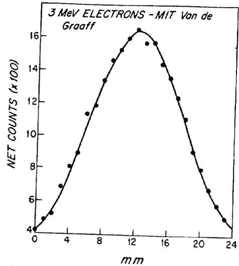
Fig. 3. Beam profile of a Van De Graaff accelerator.
